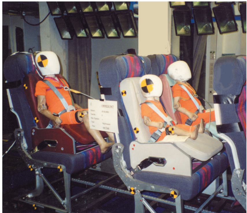
CRS – Child Restraint System • 16g dynamic test SAE AS 8049 with CRS FWD–Installation
